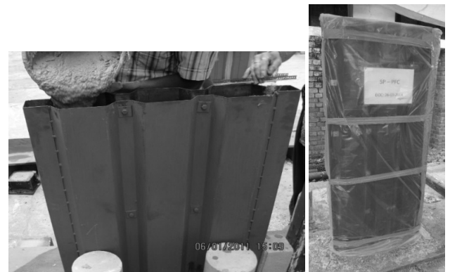
Figure 4: Casting and sealed curing of SFCC panels
