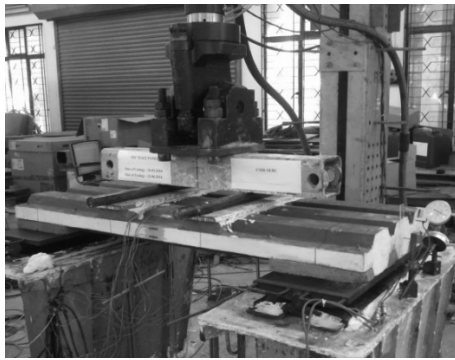
Figure 5: Experimental set-up and instrumentation: b. Flexural load (Prabha et al. 2018)
