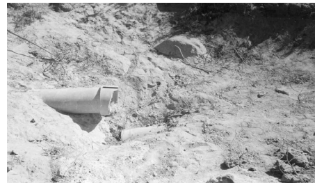
Figure 52: Failure of piping crossing the fault plane or the ground rupture during 7.6M Bhuj earthquake of 2001
