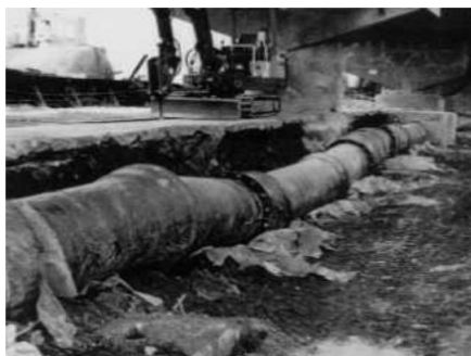
Figure 46: Buried pipelines under earthquakes - ductile iron pipes with seismic joints surviving large permanent ground deformation (left) and brittle failure of cast iron pipes (right)
