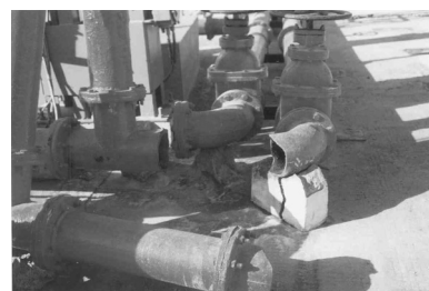
Figure 5: Two fire water lines moving on the IFFCO jetty experienced failure near the elbow as well as near the flange on the vertical branch.(7.6M, January 26, 2001, 50 km epicentral distance, 0.37 g PGA estimated)
